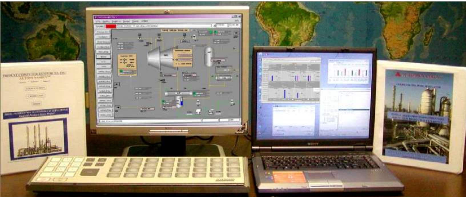
Shown with Notebook PC, Foxboro Annunciator/Numeric Keyboard, and Dual-Headed Operator Station Configuration
